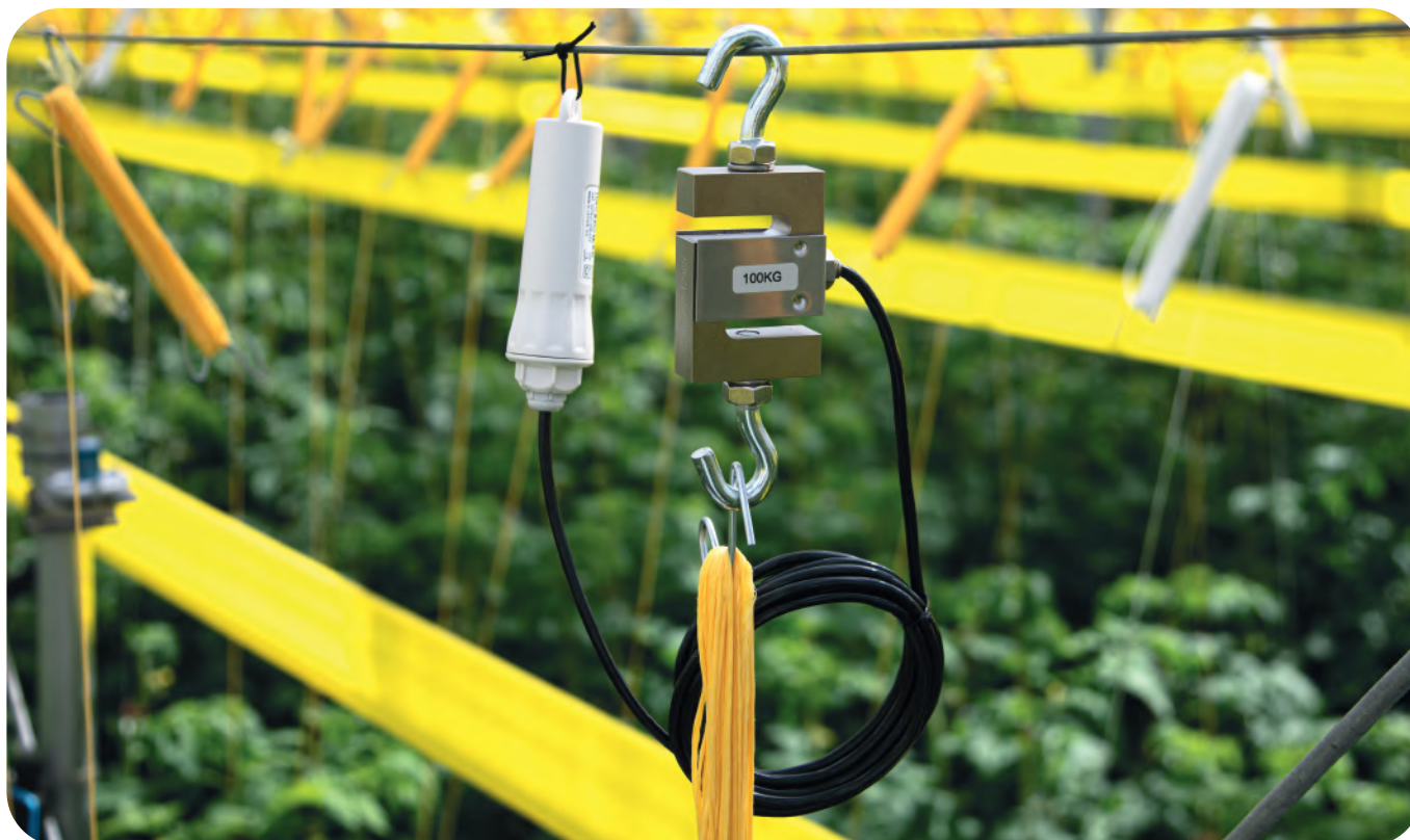
To track biomass gain, fruit load, etc, install a Weight sensor directly at the truss.
