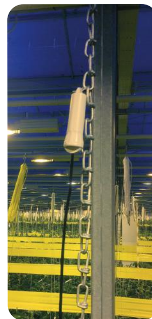
To track biomass gain, fruit load, etc, install a Weight sensor directly at the truss.
