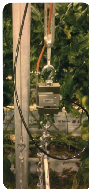
To track biomass gain, fruit load, etc, install a Weight sensor directly at the truss.
