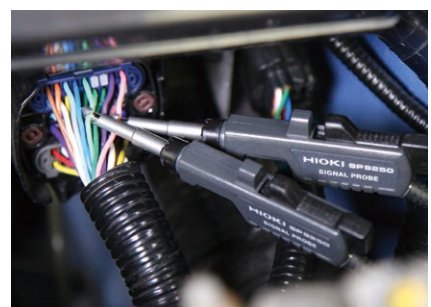
Undamaged wires for easy and safe measurement
