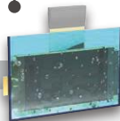
Electrolyte filling and impregnation
