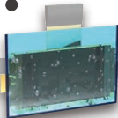
Electrolyte filling and impregnation
