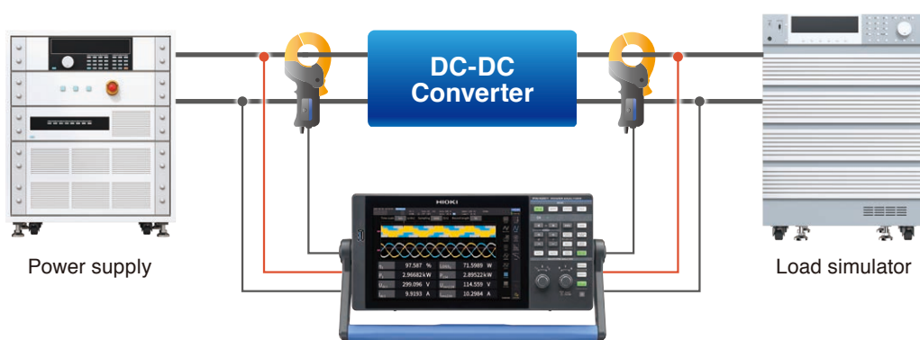
Efficiency testing in development and production
