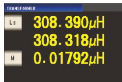
Transformer measurement mode Mutual inductance measurement screen
