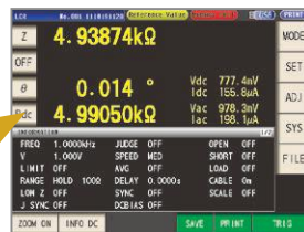
Measurement screen (LCR mode)
