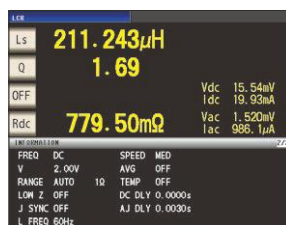
L, Q and Rdc continuous measurement screen
